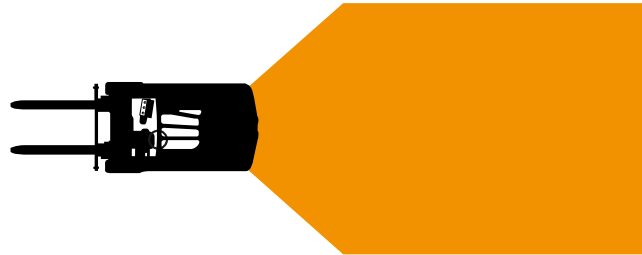
Example of configuration of a danger zone at the back of a forklift
