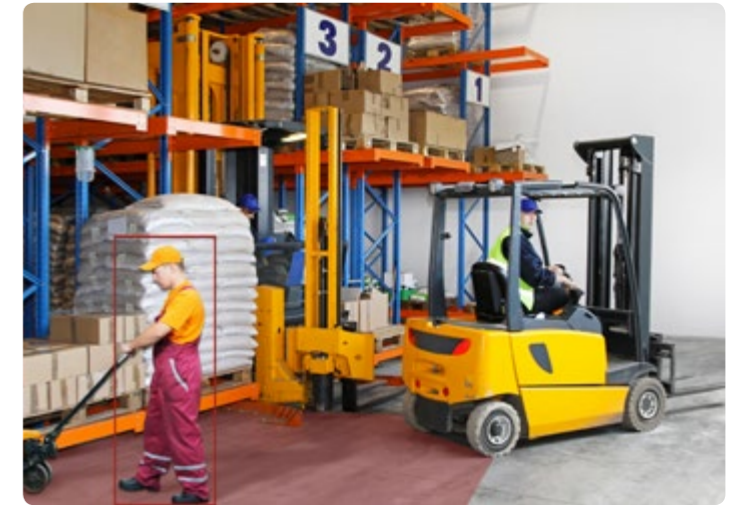
Pedestrian detection zone on a forklift - Blaxtair® recognizes all the pedestrians in its field, it warns the driver about the presence of the pedestrian in the danger zone.
